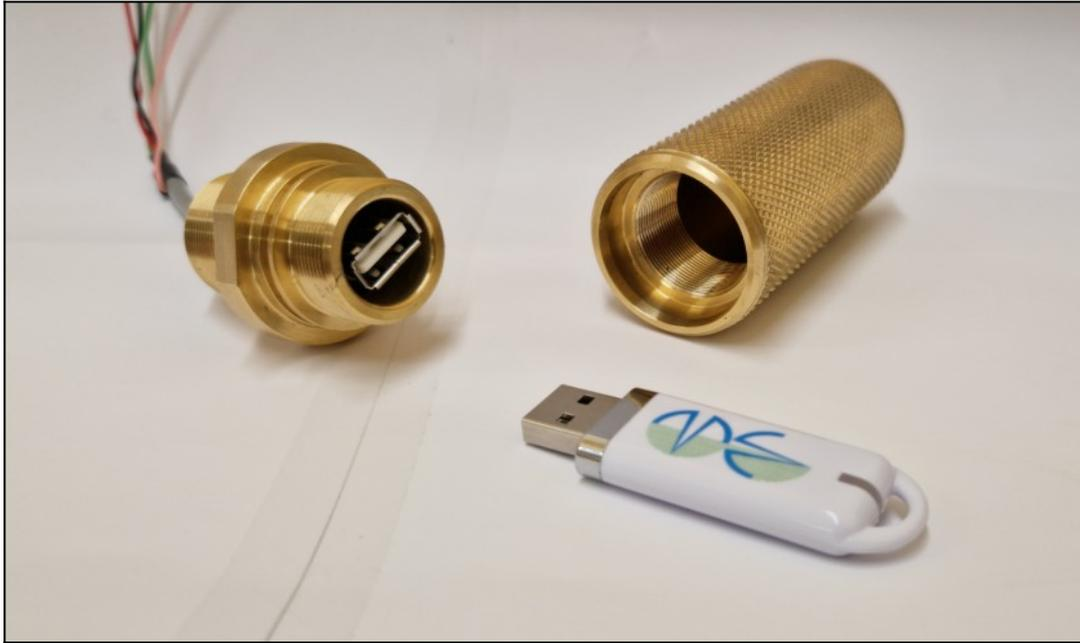
The Subsea USB Dongle enables a standard USB dongle to be fitted to subsea equipment for fast retrieval of data from the equipment without having to open the equipment and risk contaminating the sealing surfaces of the main equipment and therefore reducing the risk of flooding.
